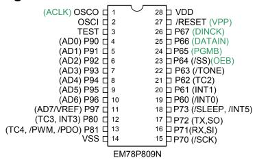
Fig. 1. Pin Assignment
